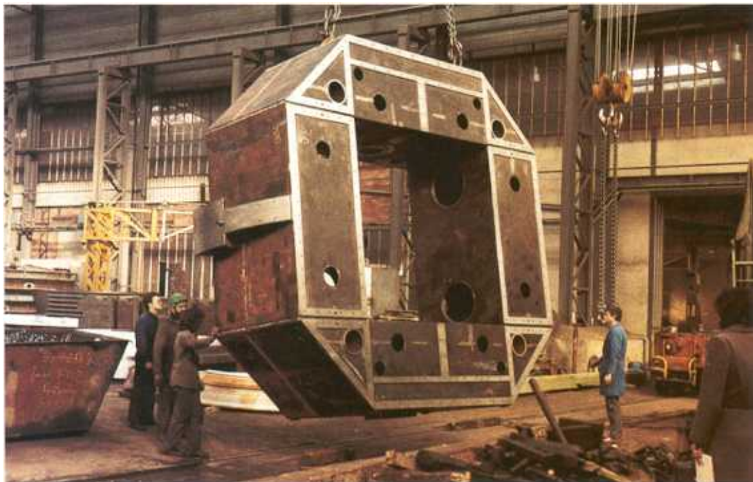
Fig.5.10: The elevation frame for the fourth antenna mount during fabrication at FERRY-CAPITAIN. This part interfaces with the central hub of the reflector.
