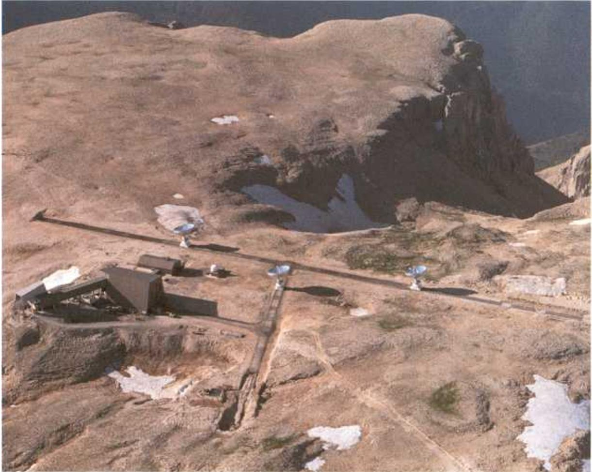
**Fig. 4.3 :** Aerial view of the Plateau de Bure in the summer of 1994 (picture taken by J.P.Wallez). The track extension work on the E-W arm is already well advanced, the extension to the North has been prepared. The new stations are fully operational since the fall of 1995.
