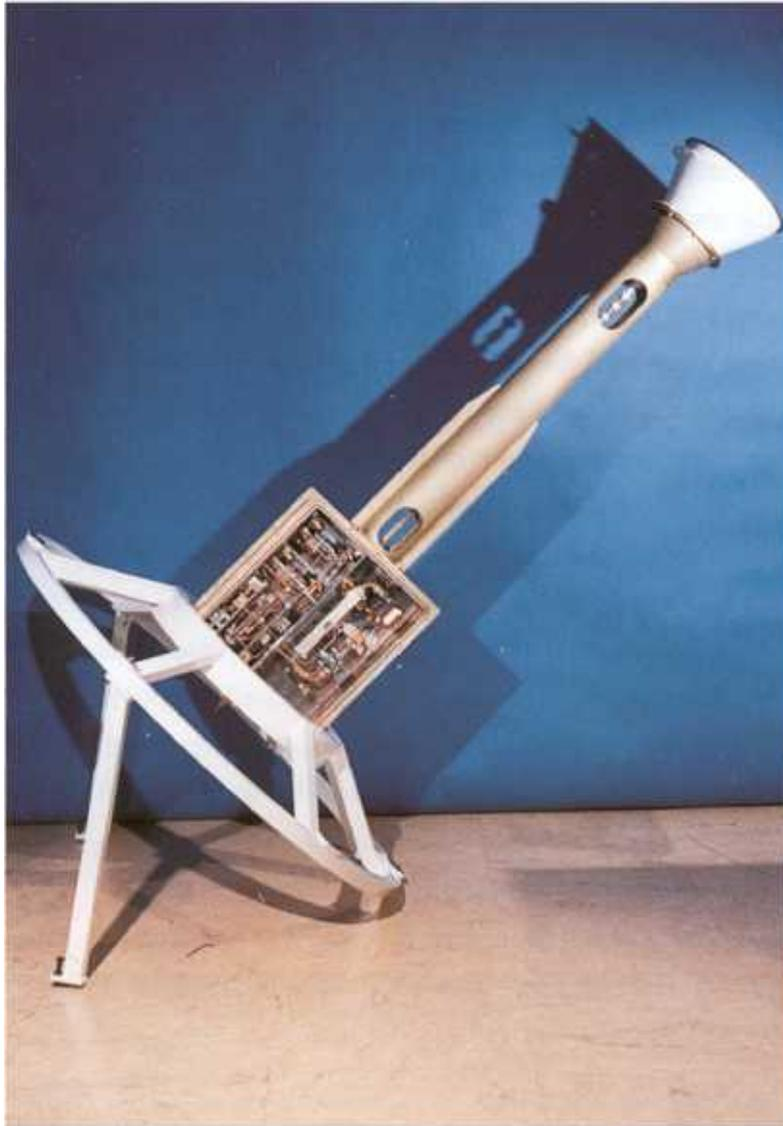
**Fig. 5.5 :** The 39 GHz holography receiver for the prime focus of the 30m-telescope. The reference horn is in the upper right corner.
