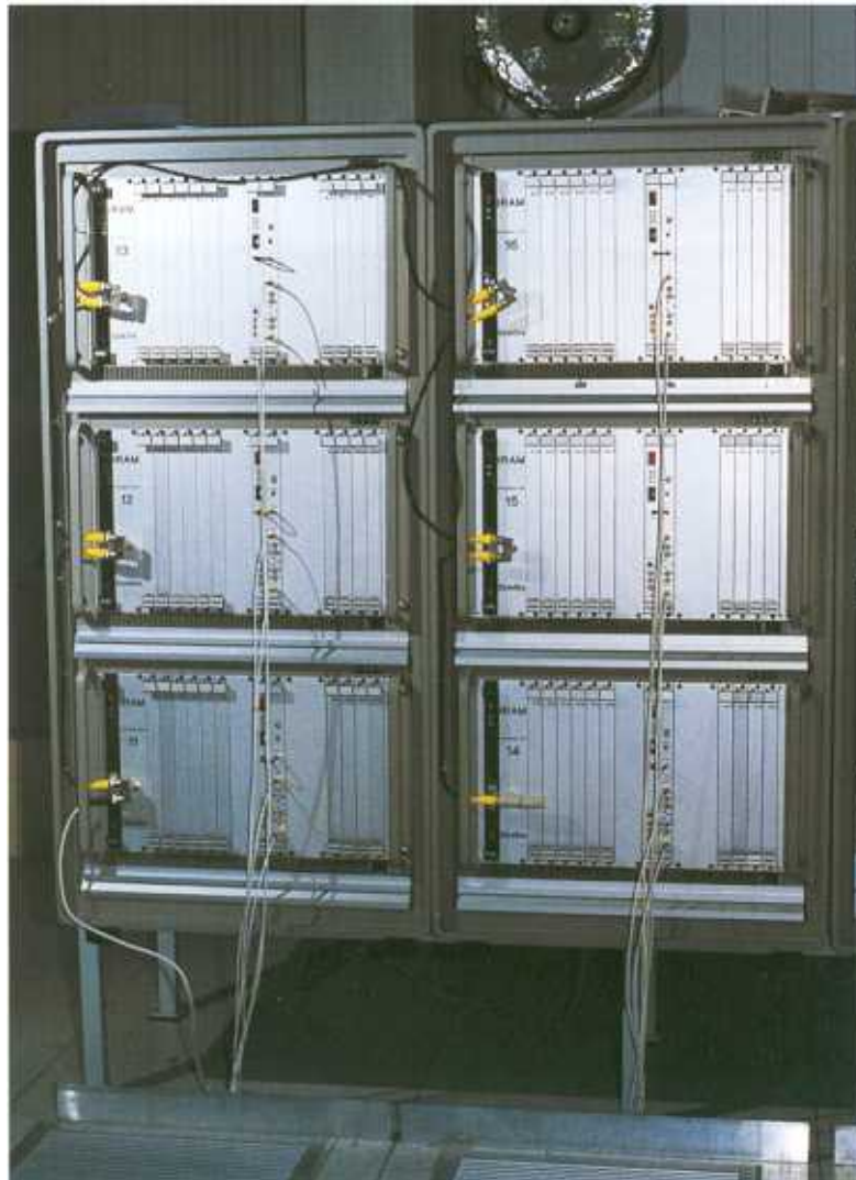
Fig. 5.8 : Block of 6 satellite correlator units receiving data from the master correlator (12 cables from the floor) at 1 Gigabit/second.
