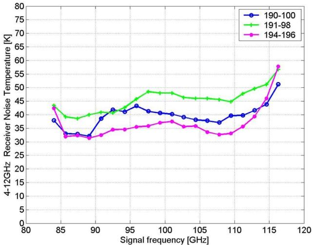
Figure 4: P. Serres et al.: Receiver noise temperature in the 84-116 GHz range, based on HEMT MMIC amplifiers.
