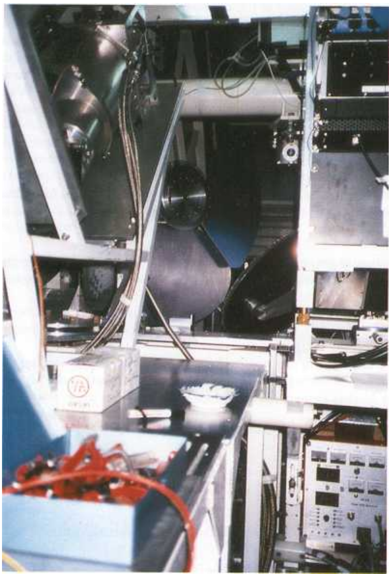
View of receiver cabin: in the center the optics, on the left the 1.3 mm receiver, and on the right the 0.8 mm receiver.
