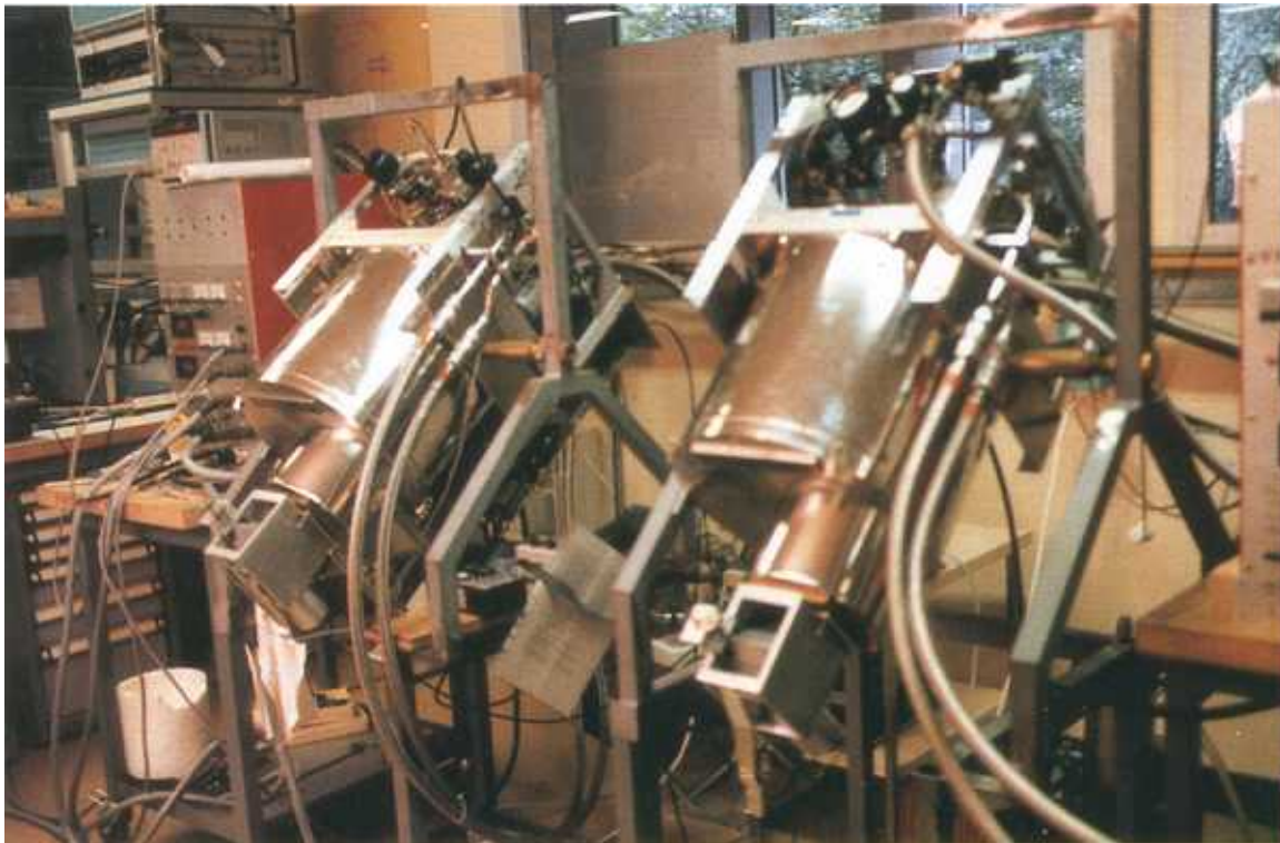
Two SIS receivers in the laboratory during the interferometer system tests.
