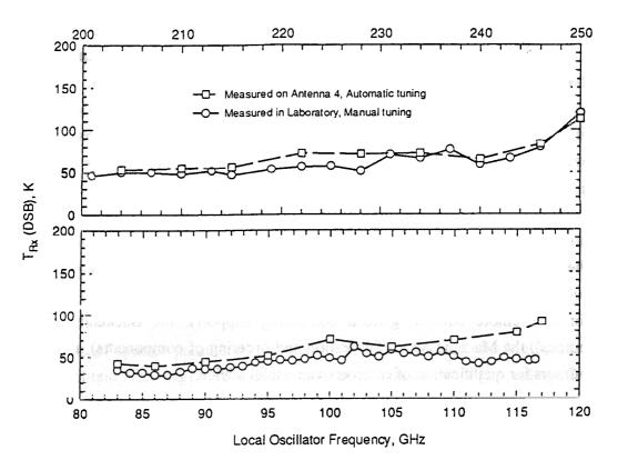
Fig. 5.2: Noise temperatures for the first 2-channel receiver on the PdBI
