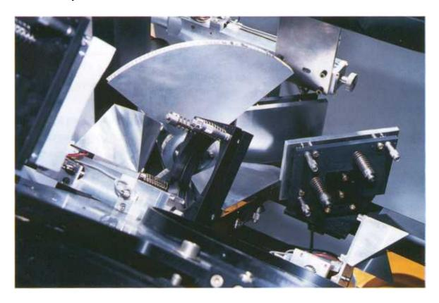
Fig. 5.12: Optical system for the dual-channel receivers. *Right to left*: hot load, mirrors, chopper, grid, cold load, and 230 GHz elliptical mirror. *Lower right*: hot load on 115 GHz input.
