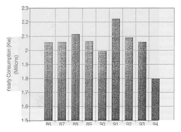
**Fig. 3.3 :** Yearly electricity consumption at the 30m telescope for the years 1986 to 1994. A reset of the antenna climatization system is now possible without stopping the observations.
