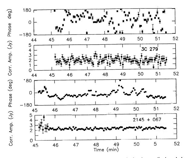
**Fig. 2.2 VLBI at 215 and 86 GHz.** Two 6.5-minute records showing amplitude and phase stability in a VLBI observation in December 1994 between Pico Veleta and Plateau de Bure. *Upper two panels:* phase and correlated amplitude at 215 GHz on 3C279. *Lower two panels:* phase and correlated amplitude at 86 GHz on 2145+067.
