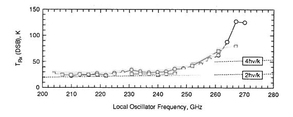
Fig. 5.9: Performance of the test receiver with two of the new 1.3 mm SIS mixers for the dualchannel receivers for the Plateau de Bure. This is the first design with a fully optimized integrated circuit.
