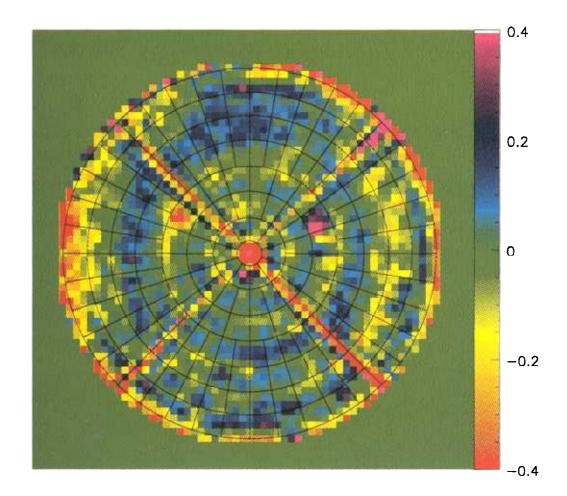
Fig. 3.4: The aperture phase distribution of the 30m telescope as derived from the November 1994 holographic measurement. The colour scale covers the range  $\pm 0.4$  radians ( $\pm 240 \mu$ m). A displaced test panel can be seen in the top right hand quadrant.
