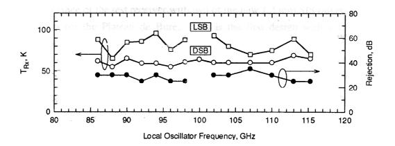
Fig. 5.8: Performance of the 3 mm receiver at the Pico Veleta telescope after installation of the new SIS mixer. Receiver noise is measured in front of the dewar.
