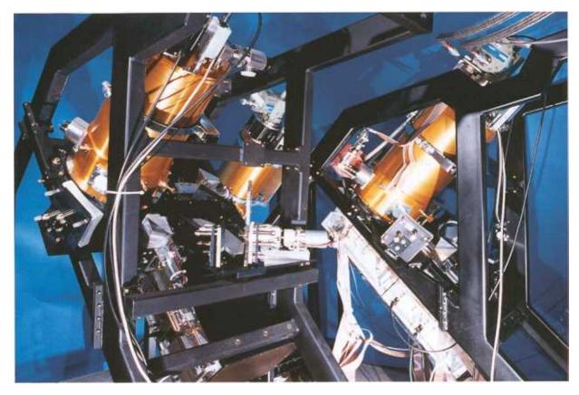
Fig. 5.3: View of 3 of the dual-channel receivers under construction. One of the systems is equipped with a beam switching chopper.
