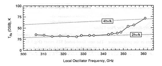
Fig. 5.5: Noise temperature of the  $\lambda 0.8$  mm receiver on the 30-m telescope.
