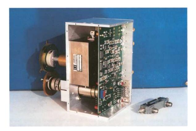
Fig. 5.11: This 1875 MHz oscillator, mounted on silent blocks, delivers an LO reference signal of high spectral purity to the PdB receivers.
