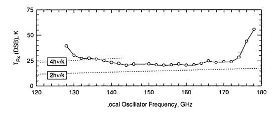
Fig. 5.10: The new fixed tuned  $\lambda$  2 mm mixer in a laboratory receiver with cooled optics with a minimum DSB receiver noise temperature of 20 K.
