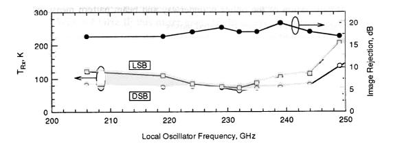
Fig. 5.7: Double- and single-sideband receiver noise temperature and image rejection for the 230 GHz (G2) receiver with the new mixer.
