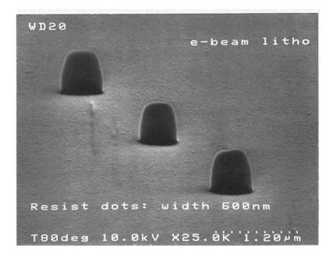
Fig.5.1: Sub-micron resist stencils for junction definition made by electron beam lithography.
