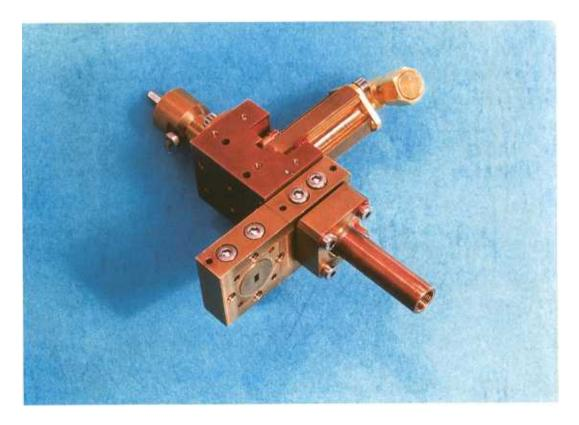
Fig. 5.4: The  $\lambda$  0.8 mm fixed-tuned SIS mixer with a corrugated horn and waveguide coupler for local oscillator injection.
