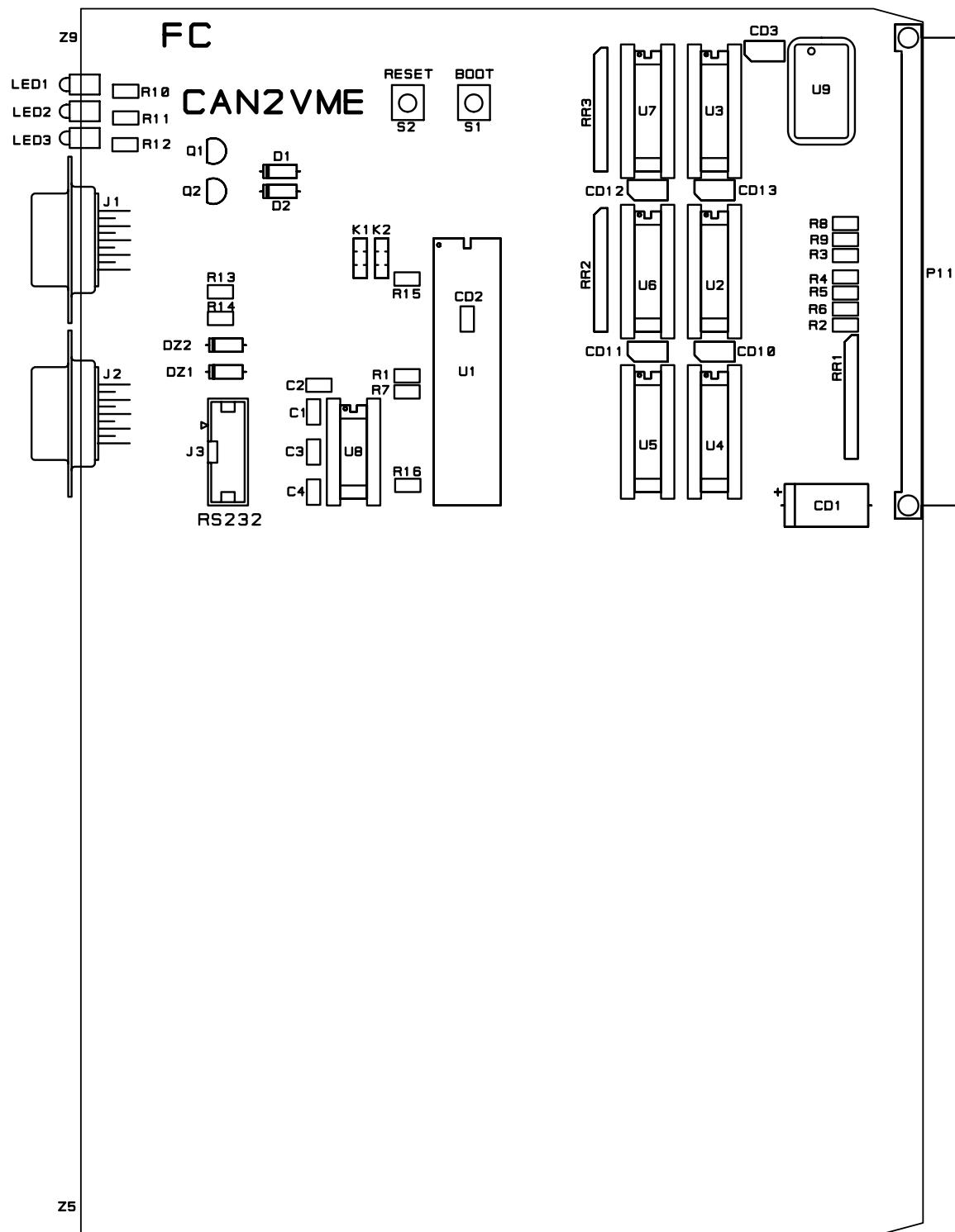
For compatibility with the VME mechanical standard, the controller is a 6U board, but it may simply be cut to 3U if necessary.
