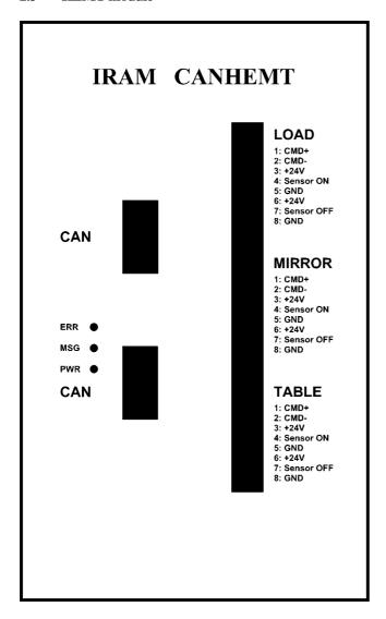
This module can be extracted from the rack and has no backplane connections. It needs 2 power supplies isolated from each other:
