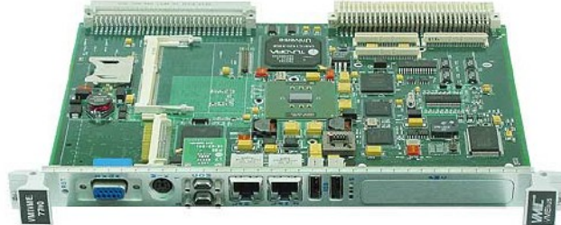
Figure 1: VMIVME-7700 from GEFanuc Automation
