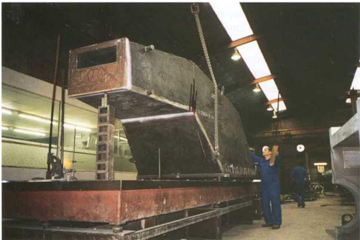
**Fig. 5.13:** Dimensional check, after welding, of a fork arm (weight 4 tons) for Antenna 5 on a marble-table at Ets. ROCHE at Reims.
