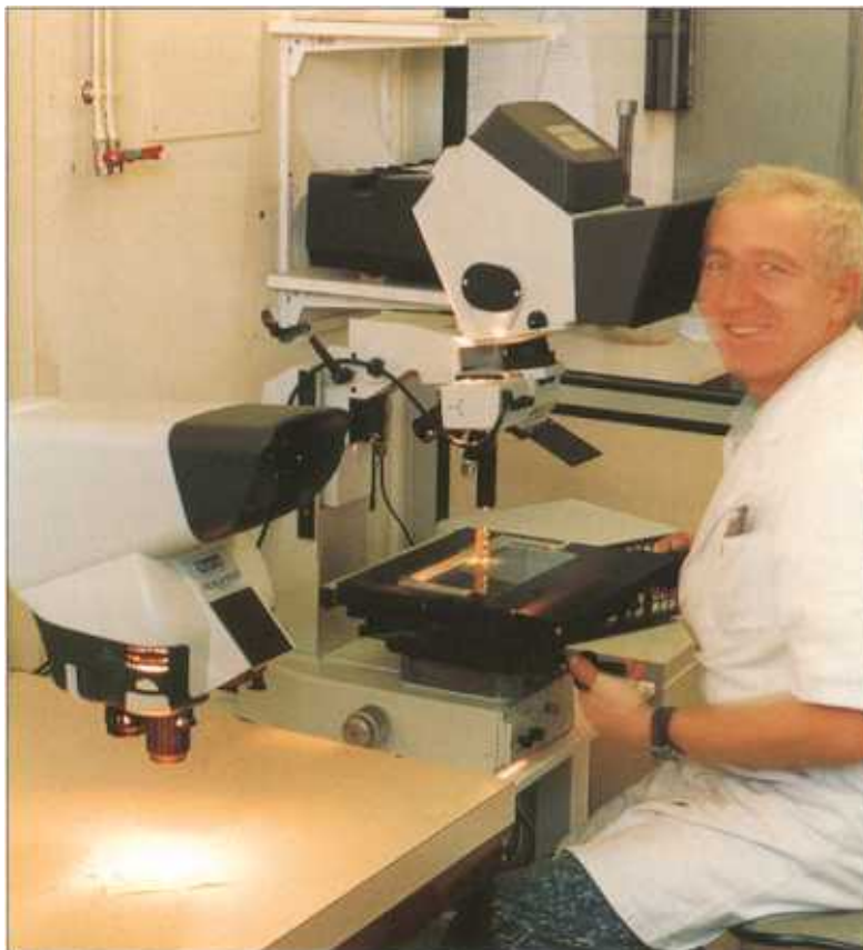
Fig. 5.6 : Quality control of micro-machined components. This device allows measurements with an accuracy of \pm 1 \mu\text{m} in xvz.
