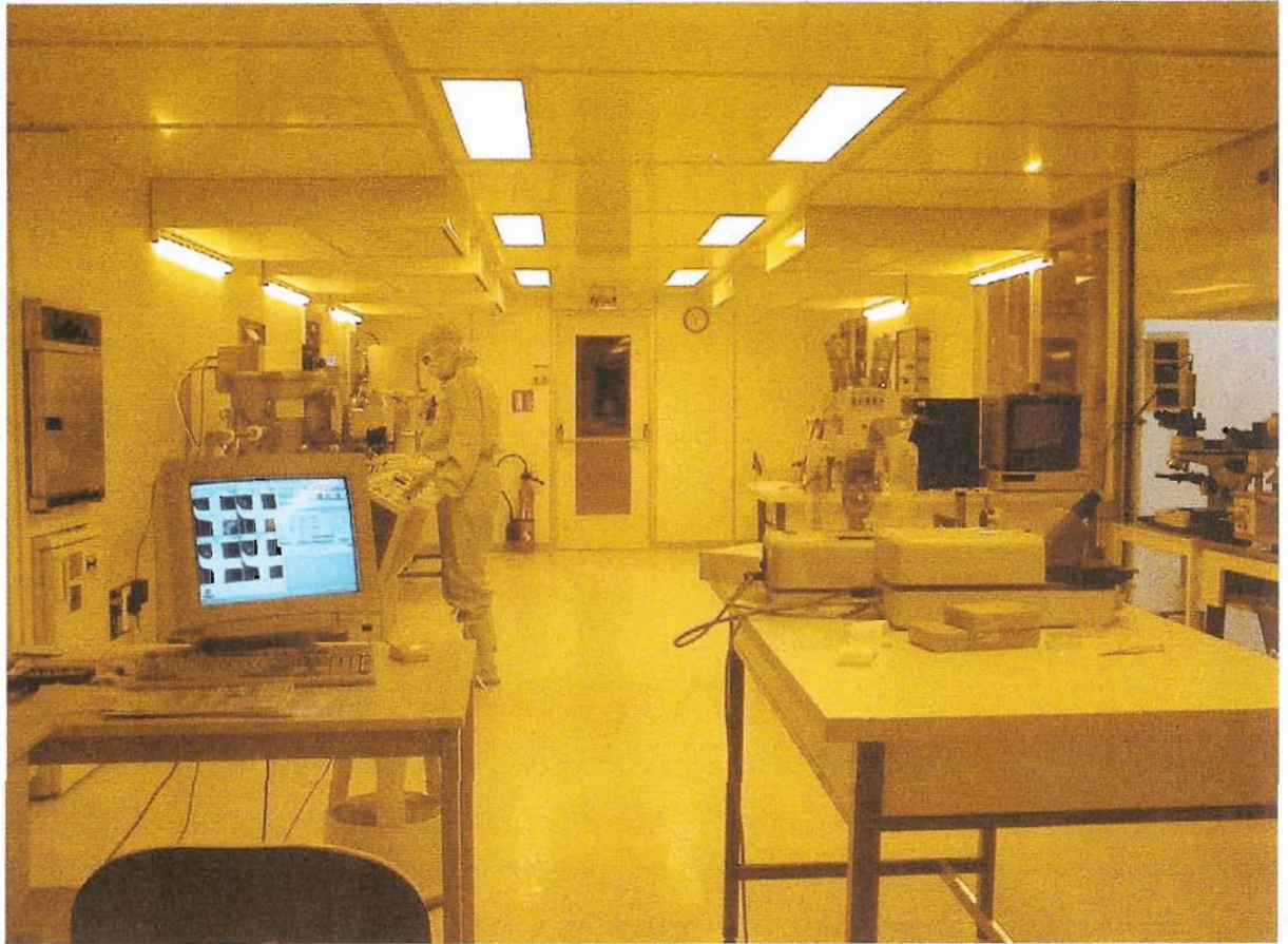
Fig. 5.1 : The new IRAM clean room for processing of superconducting devices.
