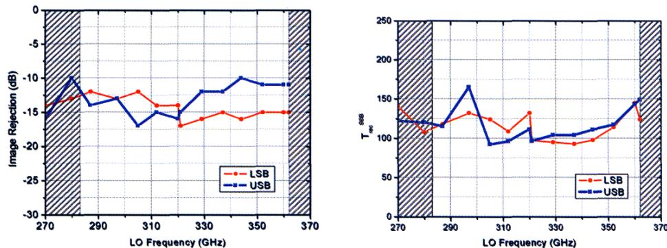
**Fig. 5.9:** Results obtained with the prototype sideband separating mixer for ALMA band 7. Left: image band rejection; right: (quasi-)SSB noise temperature in a narrowband IF.
