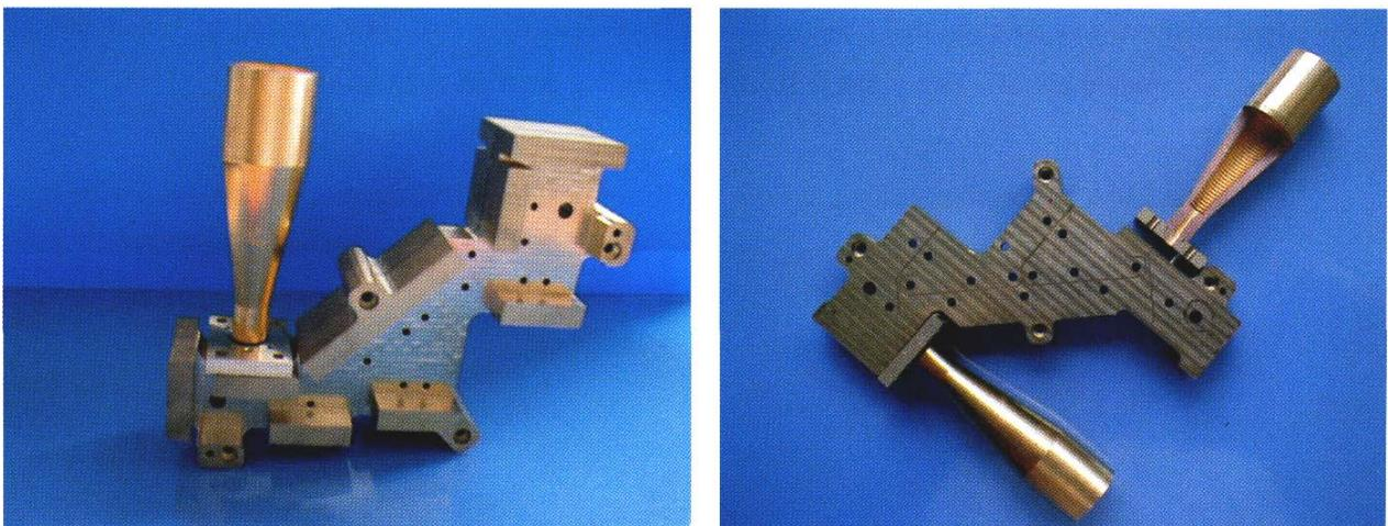
**Fig. 5.13:** 230 GHz couplers fabricated by the IRAM workshop staff
