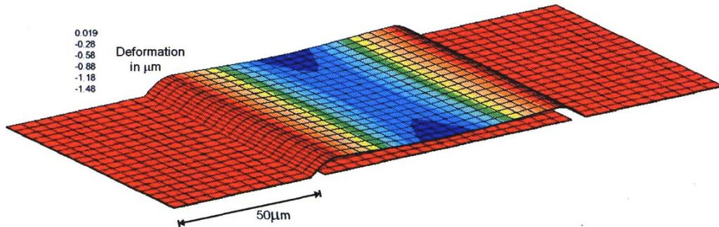
**Fig. 5.3:** Finite element simulation of a variable capacitance air bridge system from Niobium with an applied voltage of 80V. The calculation clearly shows the necessity of 3-D modeling.
