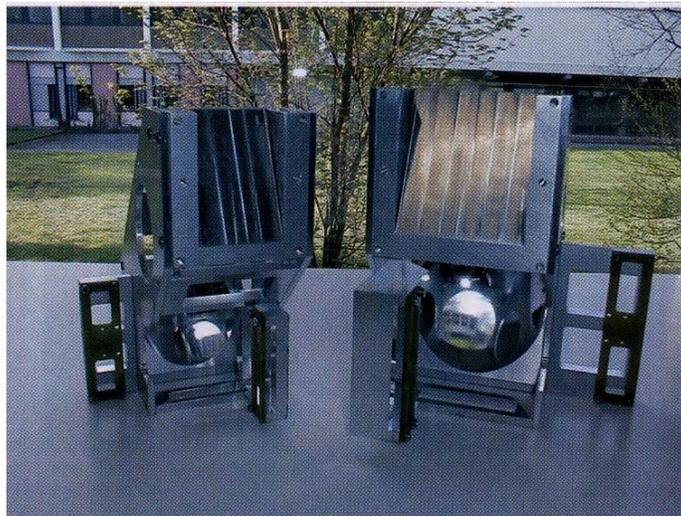
**Fig. 5.7:** Prototype optics modules (two elliptical mirrors each) for PdB bands 1 (83-117GHz) and 3 (200-260GHz).
