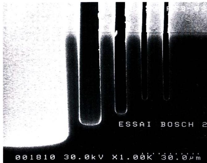
**Fig. 5.2:** Test pattern of Si micro machining with the new Alcatel ICP equipment
