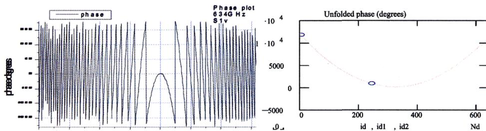
**Fig.5.11:** Phase pattern of a prototype feed for ALMA band 9. Left: phase modulo  $2\pi$ ; right: unfolded phase, showing that coherent measurements could be made up to the edge of the pattern, where the amplitude is -30dB from boresight. The measurements have been carried out together with a SRON team from Groningen.
