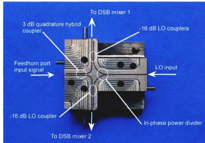
**Fig. 5.8:** The combination of quadrature hybrid, LO power splitter, and LO injection couplers that is the central element of the prototype sideband separating mixer for ALMA band 7.
