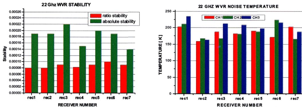
**Fig. 5.5:** Summary of laboratory tests of the seven 22GHz water vapor radiometers.
