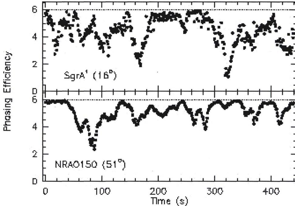
**Fig. 4.4** : Results from the VLBI observations that involved the PdB Interferometer for the first time as a phased array. The figure shows over a period of 7.5 minutes the phasing efficiencies at 3 mm for the source SgrA\*, at 16 degrees elevation, and for the QSO NRAO150, at 51 degree elevation. In the absence of atmospheric phase noise, the efficiency would be 6 according to the 6 antennas being phased.
