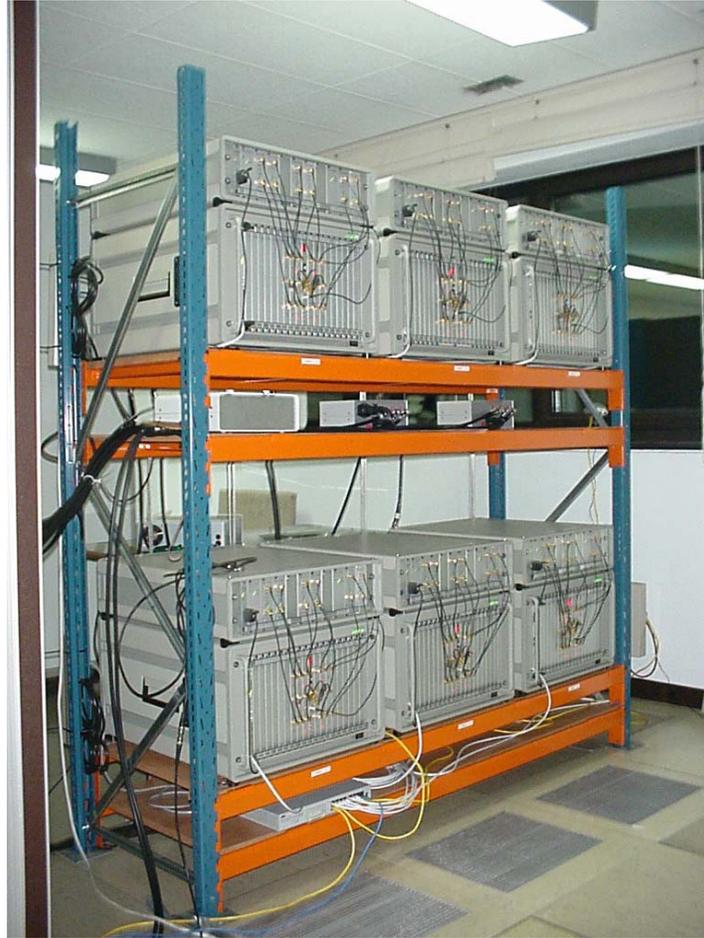
**Figure 3.7:** VESPA in the backend room at the 30m telescope. This correlation spectrometer consists of 6 units, each having a digital chassis with 12 correlator boards and an analog chassis with 15 RF modules.
