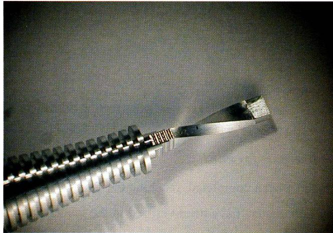
**Fig. 5.6:** Detail of new horn type with integrated waveguide twist and step transition. The twisted waveguide has dimensions 2.54mm x 1.27mm.
