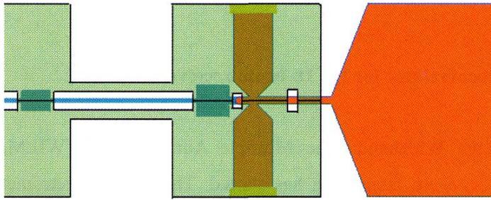
**Fig.5.10:** Layout of one of the low-capacitance mixer chips (detail). This design incorporates (besides the junction) striplines, coplanar lines, suspended striplines, shorted tuning stubs, with a total of three metallization layers.
