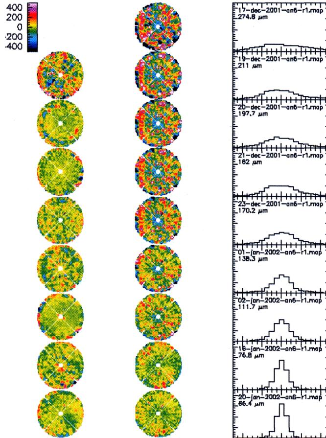
**Fig. 4.6:** Surface accuracy achieved on Antenna 6 since December 17, 2001 and after seven holography iterations: panel corrections after each iteration (left column), panel distribution according to holography results (central column), surface rms (right column).
