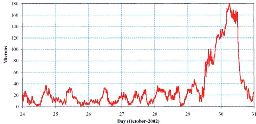
**Fig. 3.4:** The amplitude of the computed astigmatism of the antenna during five days of good weather (note that these values are larger than the actual rms). Up to day 29 the new temperature control system (TCS) was activated, from day 29 onwards it was deliberately switched off to show the effect of the old TCS.
