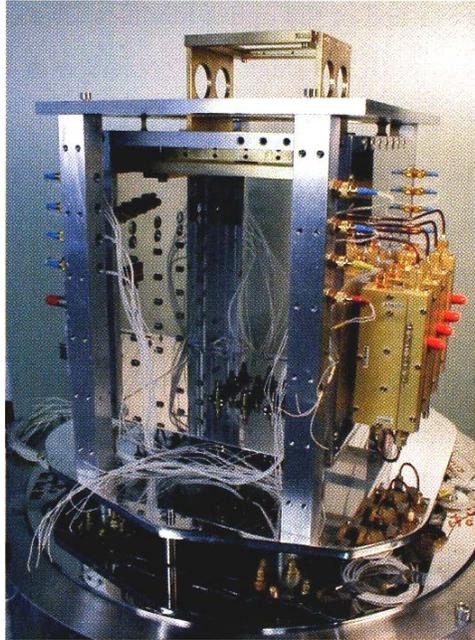
**Fig. 5.4:** The nine-pixel RF module for the second polarization of HERA during construction.
