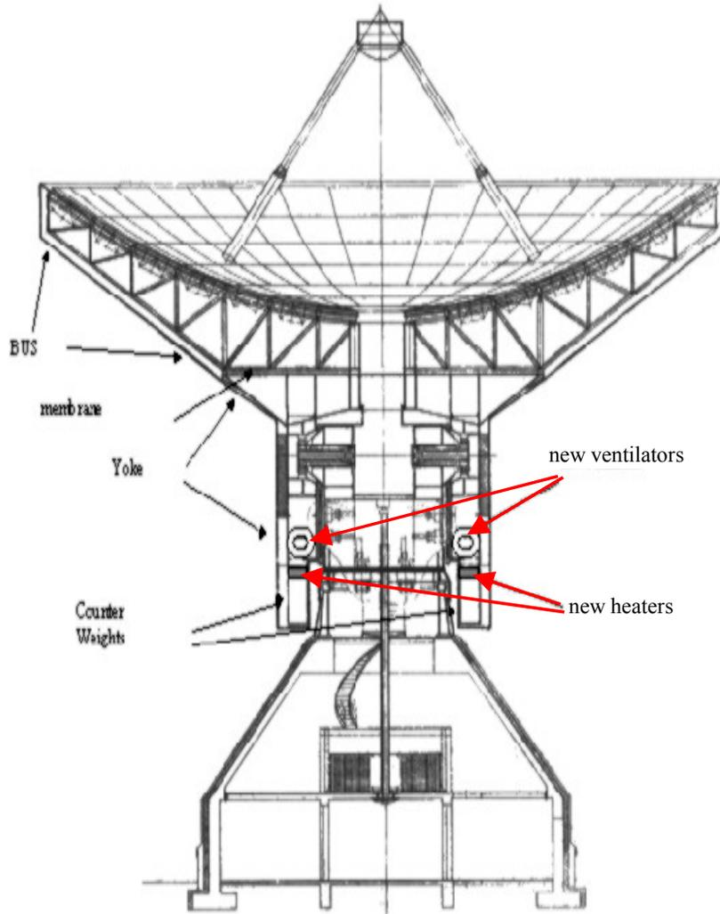
**Fig. 3.3:** Location of the added heating and ventilation elements in the 30-m telescope.
