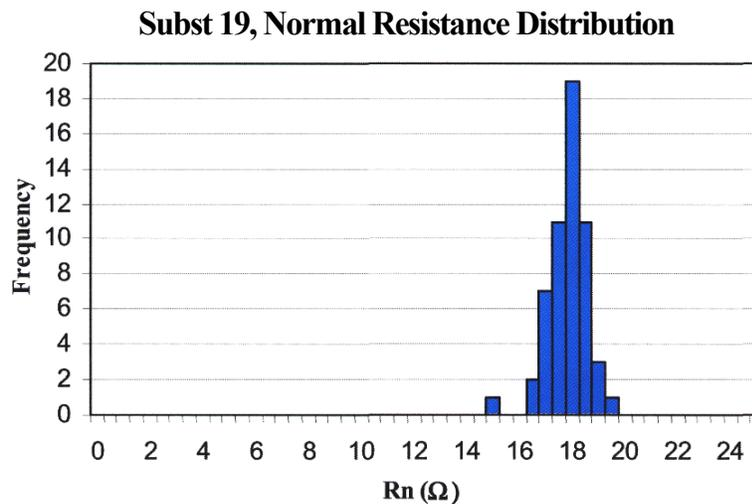
**Fig. 5.1:** Statistical distribution of the normal resistance of devices including two  $\text{lum}^2$  junctions in parallel. Under the assumption that the spread is entirely due to size variations an area homogeneity of better than 7% or a linear dimension variation of 35 nm can be derived.
