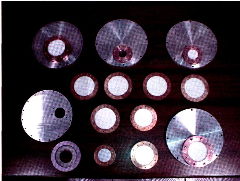
**Fig. 3.6:** Windows and IR filters for ALMA receivers.
