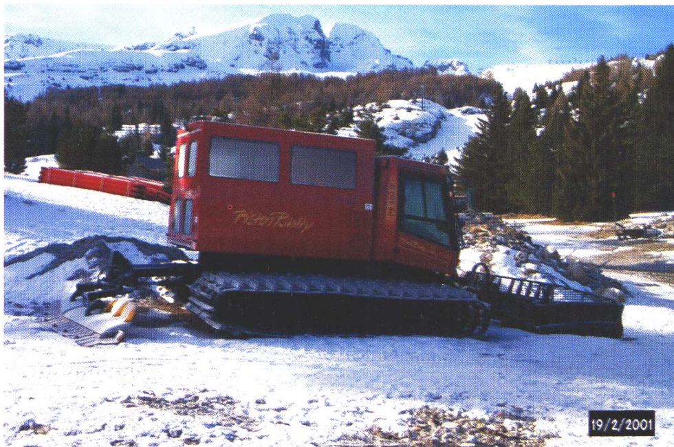
Fig. 4.1 The ratrack that has been bought to transport IRAM staff between Superdevoluy and the Sommarel area in winter time. The cabin can accommodate 6-8 passengers. It is operated by staff from the ski station, under contract with IRAM.
