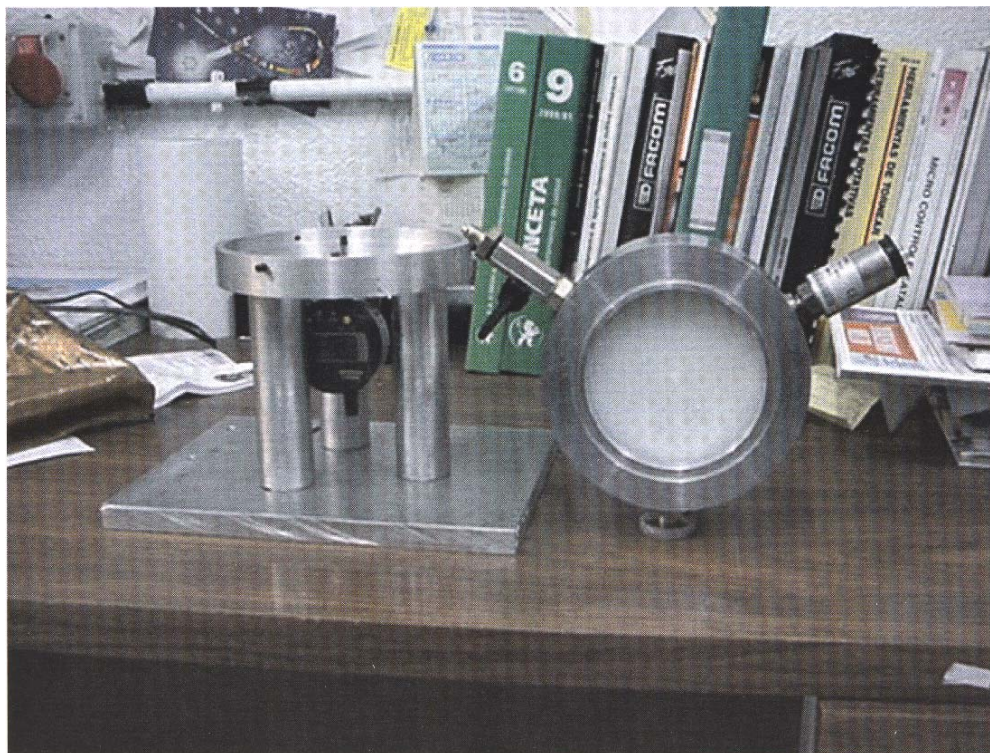
Fig. 3.4. Burst chamber constructed at IRAM Granada for mechanical and leak rate tests of vacuum window materials for the ALMA project
