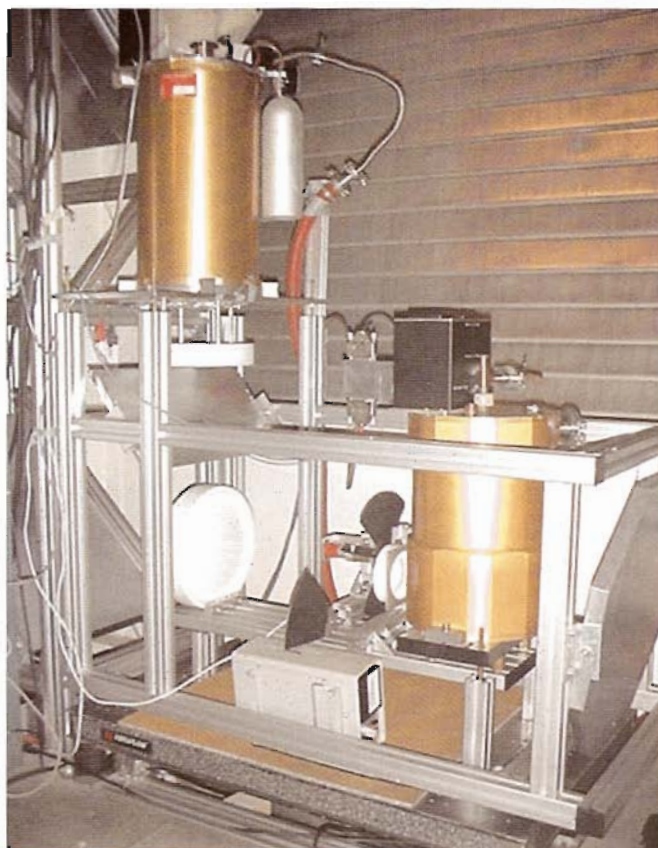
Fig. 3.5: The MAMBO I and II bolometers at the 30-m telescope
