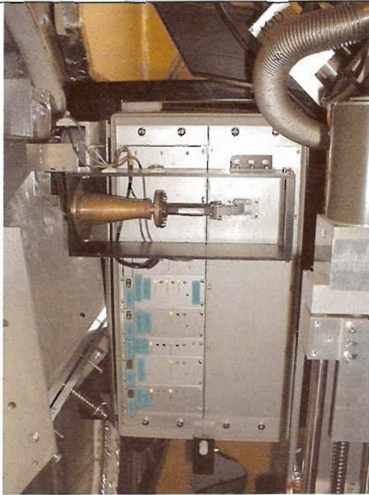
Fig. 5.7: The first 22 GHz water vapor radiometer installed on site. This receiver is located to the side of the SIS receiver. The corrugated horn is coupled to the telescope via a pair of mirrors (elliptical, flat), partly visible on the left of the picture.
