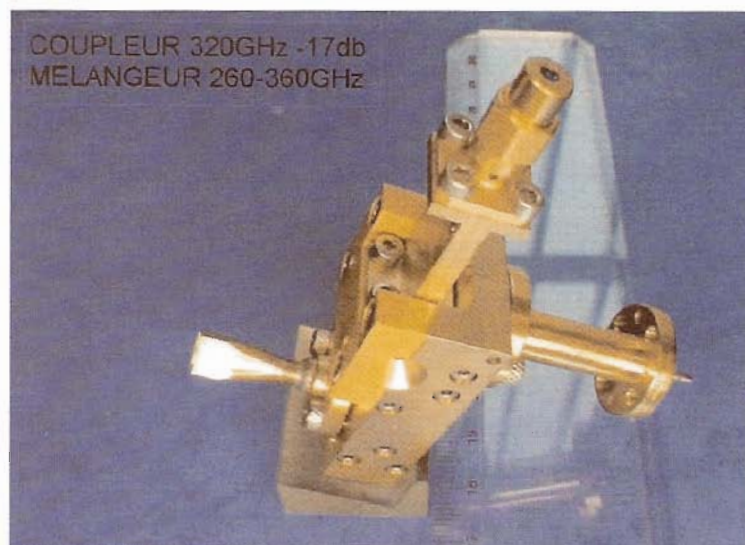
Fig. 5.13: Assembled coupler and mixer block for the ALMA band 7
