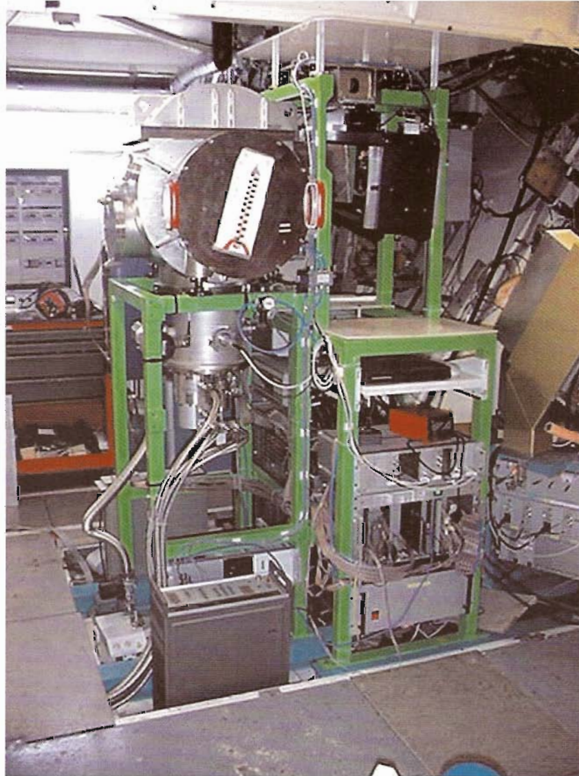
Fig. 3.4: HERA, a 9 pixel receiver for 230 GHz spectroscopy. In a second step it will be equipped with 18 channels.
