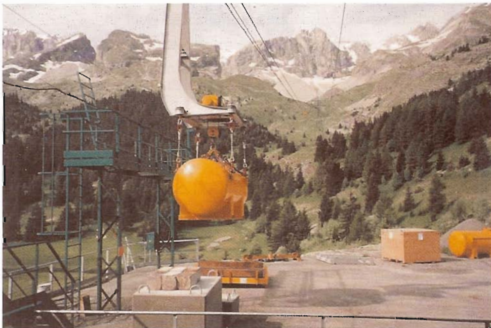
Fig. 5.15: The picture shows a newly constructed container for the transport of liquids during a test with the rebuilt cable car.
