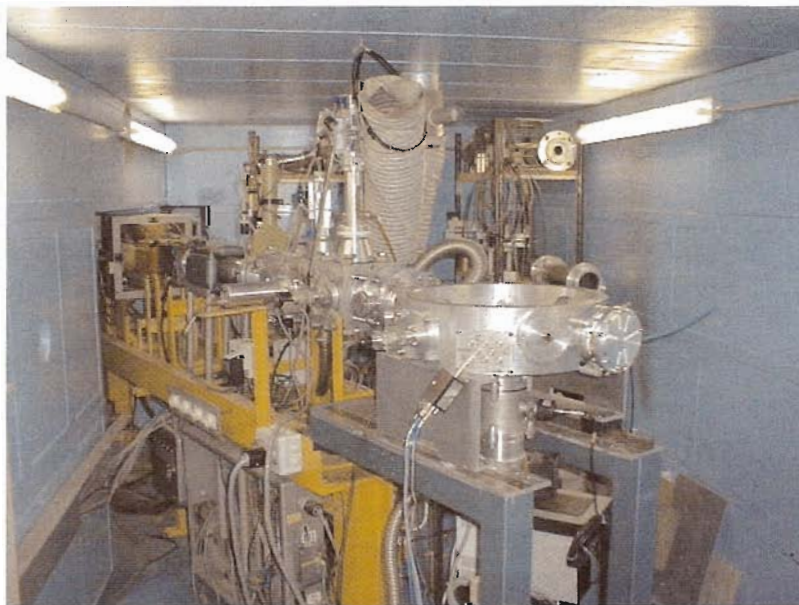
Fig. 5.1: The CERI 10MeV Proton beam line as used for radiation hardness tests for SIS junctions. The cylindrical piece in the foreground is the sample vacuum chamber containing a Rutherford disperser, the sample stage and the semiconductor reference counter.
