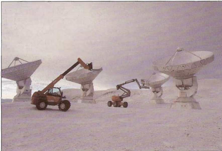
Fig. 4.5: Four of the six antennas of the Plateau de Bure array. A mobile telescopic fork-lift (left foreground) and an articulated platform for aerial repair work (centre) were purchased for outdoor activities at the Observatory.
