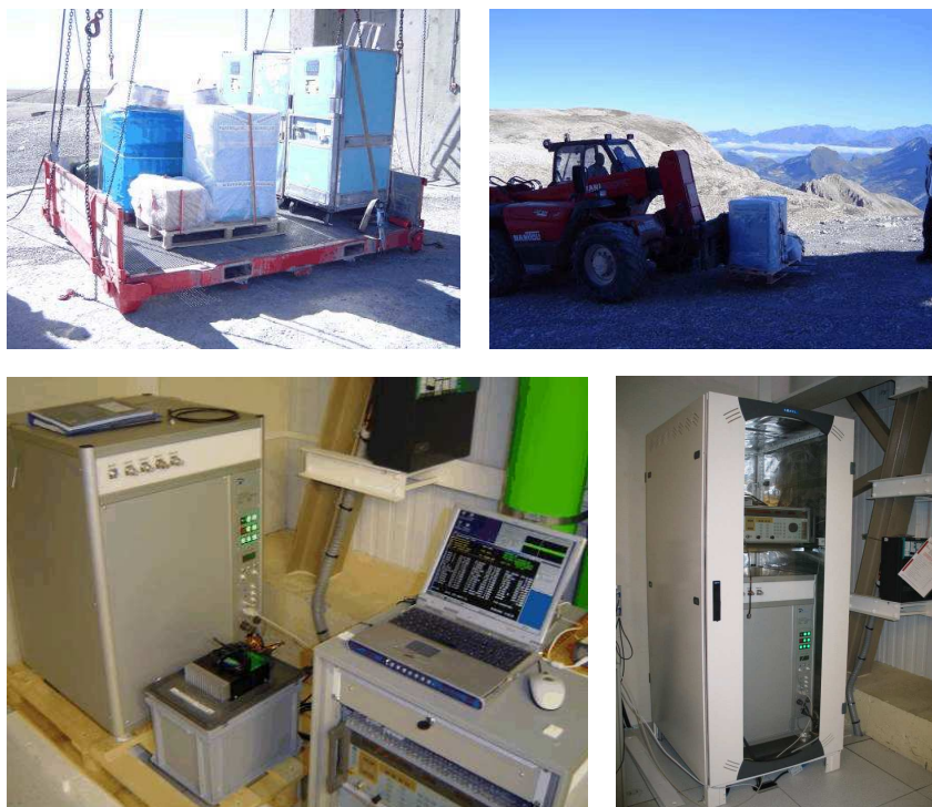
Figure 2: Arrival of EFOS-38 on the Plateau de Bure. After a transport by road, the maser was lifted by cablecar to the Plateau de Bure and then carefully moved to the correlator room where it was fully activated. The last photo shows the thermally regulated rack into which the maser was integrated in February 2007 (last photo by A. Grosz, others by M. Bremer).
