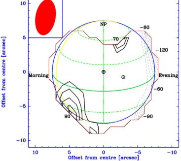
Winds near 50 km altitude in the atmosphere of Mars determined from IRAM Plateau de Bure observations of CO 1-0 lines in May 1999. Positive values indicate receding winds. Contours are separated by 15 m/s [Moreno et al. 1999]
