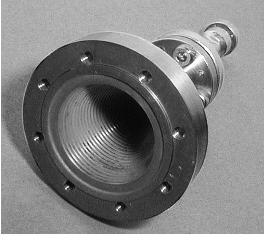
Figure 5.3: A corrugated horn for the 150GHz band. The phase-correcting lens normally present at the aperture has been removed to reveal the corrugations. The diameter of the aperture is about that of a typical coin (1DM/100Ptas/1F). All the waves collected by the 30-m antenna converge to the horn with a precise phase relationship and are then squeezed into a waveguide 2 x 1 mm across. The ratio of areas is three hundred million!
