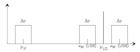
Relation between the IF, RF and local oscillator frequencies in an heterodyne system
