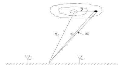
Position vectors used for the expression of the interferometer response to an extended source, schematically represented by the iso-contours of the sky brightness distribution.
