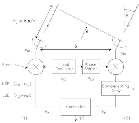
2-element heterodyne interferometer with delay tracking after frequency conversion
