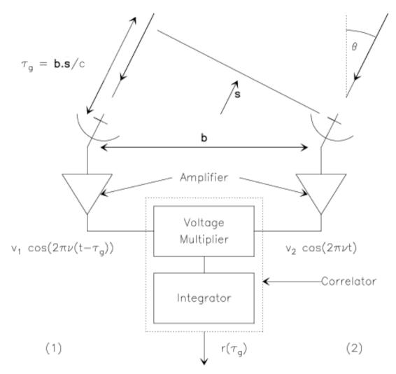
Schematic diagram of the two-antenna radio interferometer.  $\tau_g = \mathbf{b}.\mathbf{s}/c$  is called the geometrical delay
