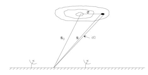
Position vectors used for the expression of the interferometer response to an extended source, schematically represented by the iso-contours of the sky brightness distribution.
