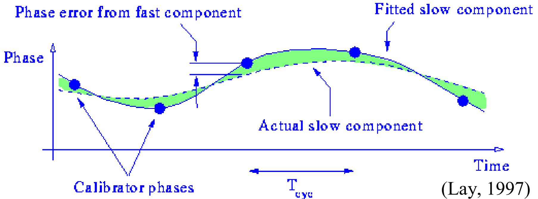
Phase is sampled at intervals  $T_c \rightarrow$  fit is sensitive to errors due to the presence of the fast component ( $< 2T_c$ ), which can be large
