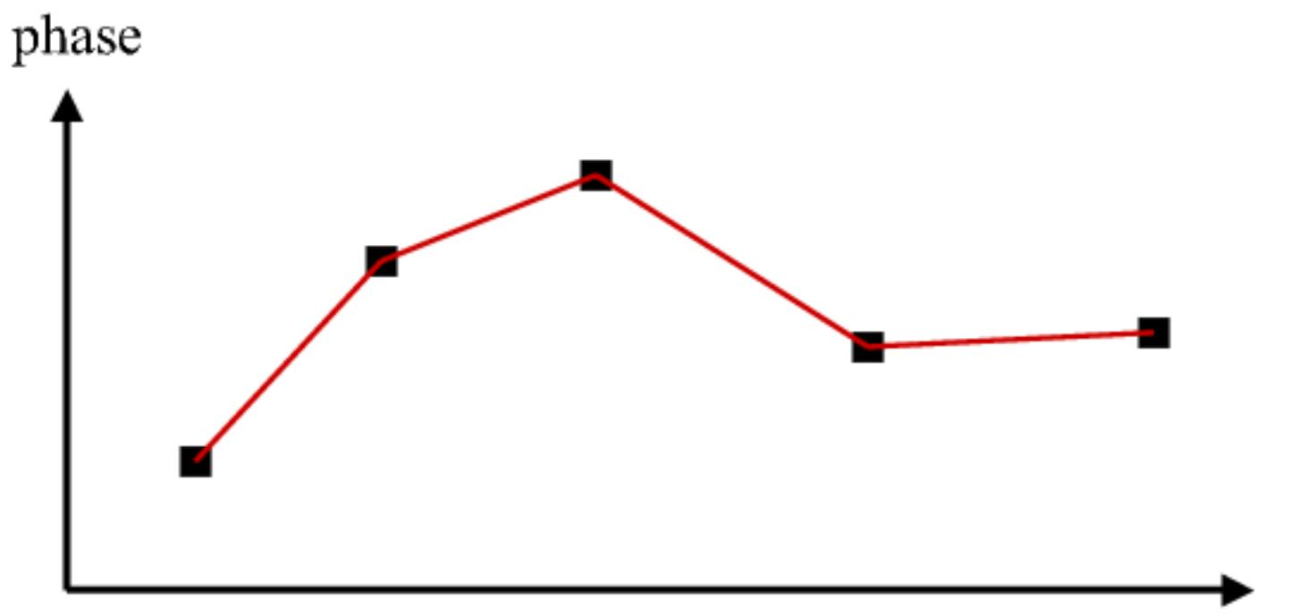
Calibration at series of points + linear interpolation
