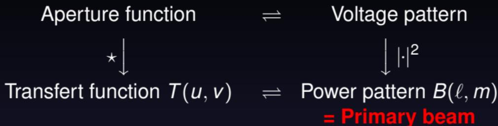
Gaussian illumination  $\Rightarrow$  to a good approximation,  $B$  is a Gaussian of  $1.2 \lambda/D$  FWHM
