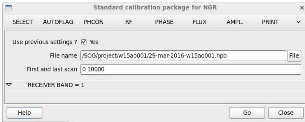
**Phase:** Remove instrumental phases in time by observing a close point-like source (phase=0).
