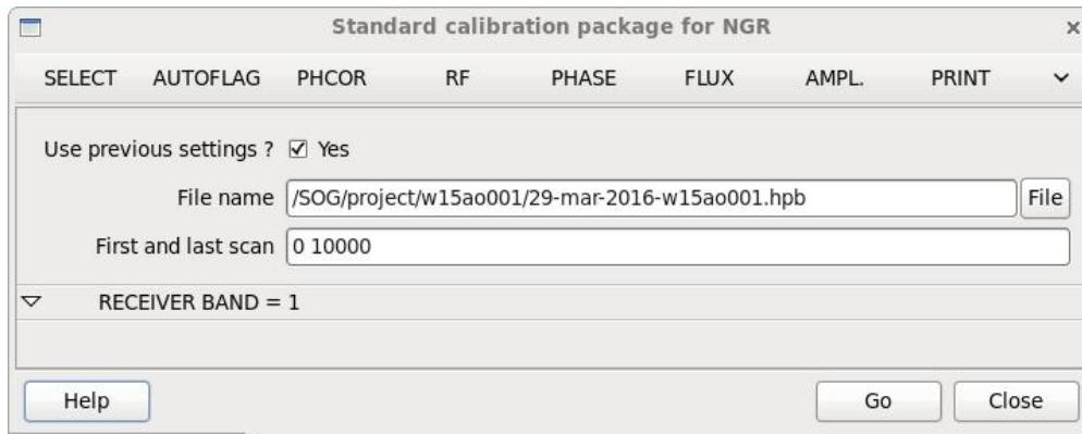
**Ampl:** Remove instrumental amplitudes in time by observing a close point-like source (constant amplitude).
