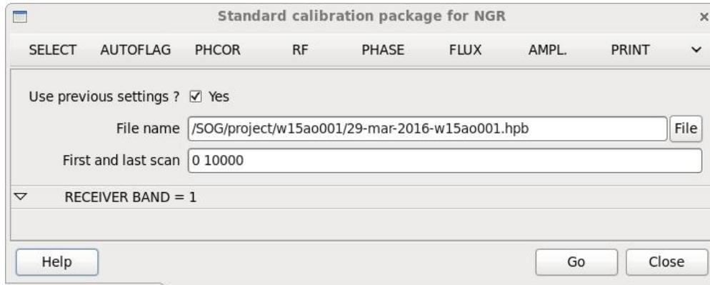
**RF:** Measure the receiver bandpass (RF) to calibrate the source data, for every spectral calibration unit (narrow and widex) and tuning (gain) range.
