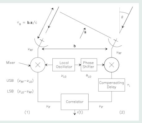
• A compensating delay is introduced in one of the branch of the interferometer, **on the IF signal**
