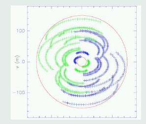
Measurements = uv plane sampling  $\times$  visibilities After FT: dirty map = dirty beam \* (prim. beam  $\times$  sky)
