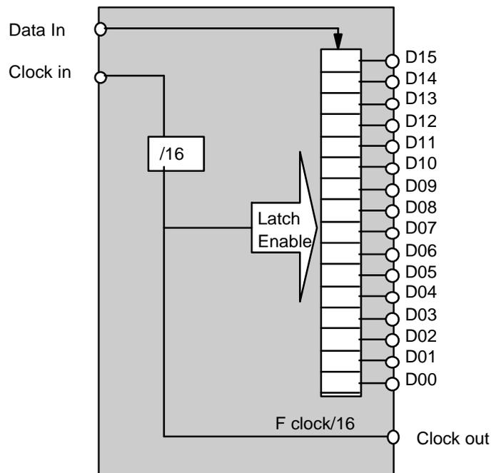
Fig.1 : Generic functional diagram of a commercial demultiplexer
