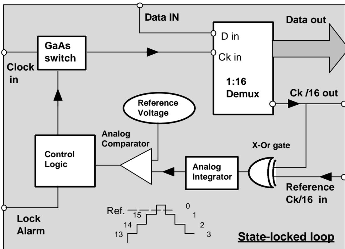
Fig 2. Block diagram of the loop
