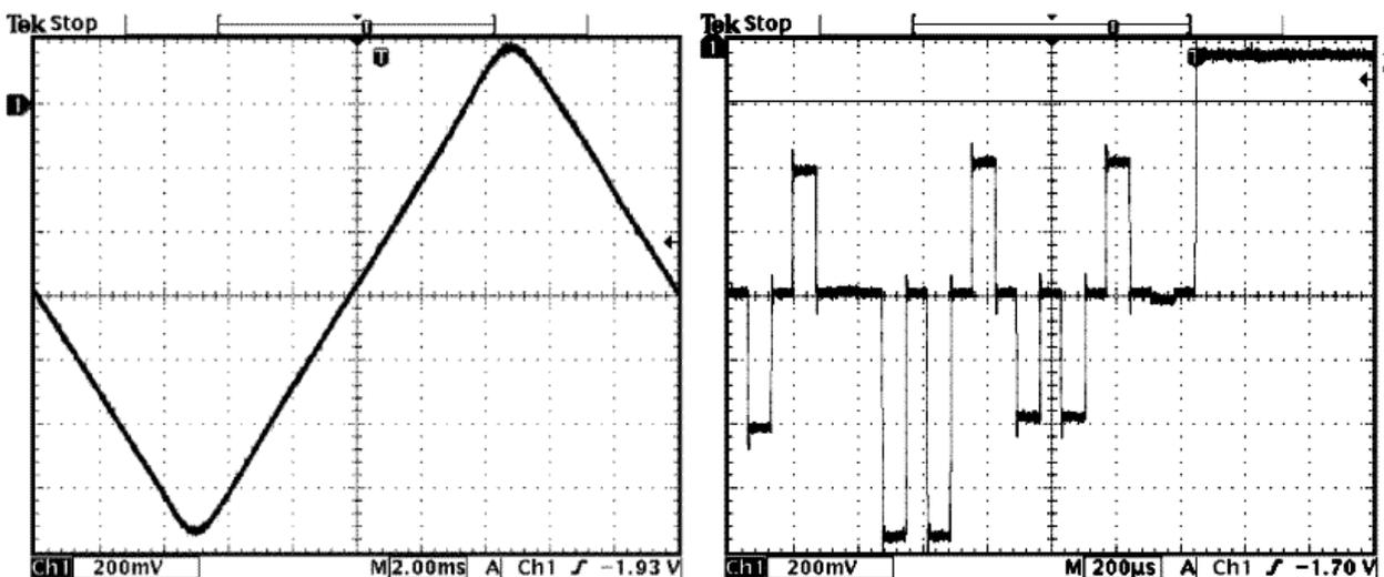
Fig 4. Outputs of the phase comparator
