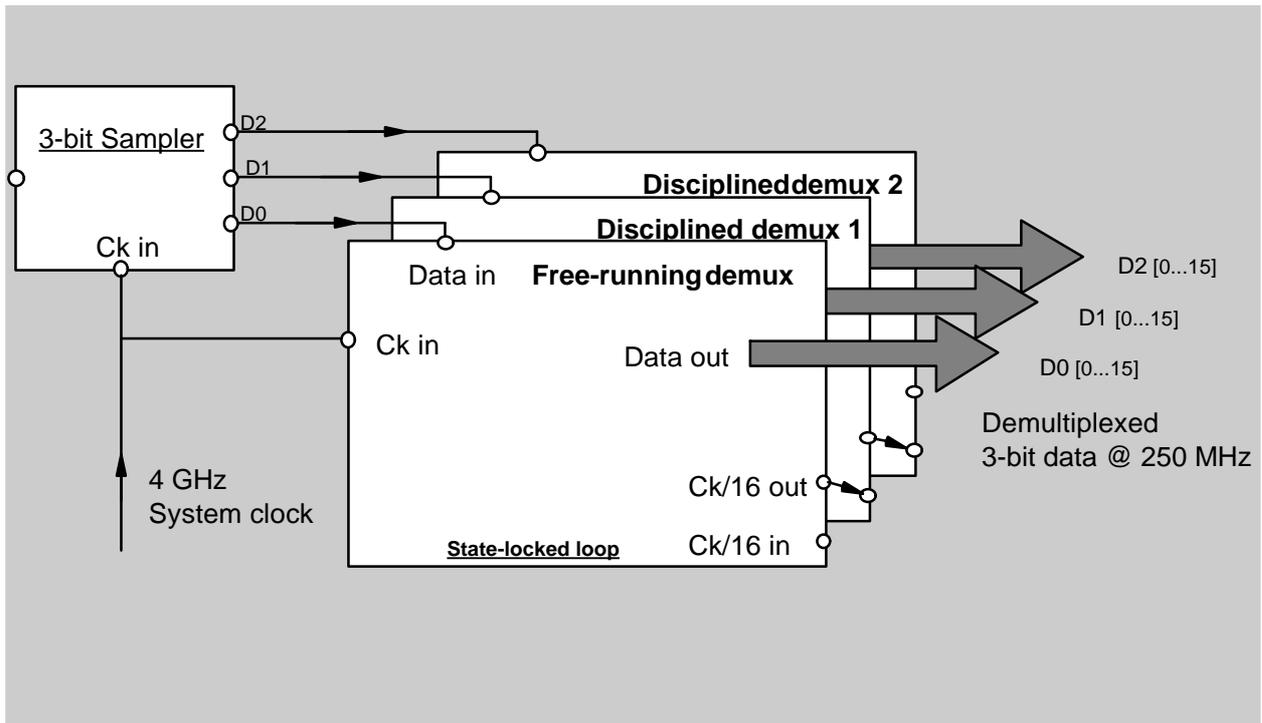
Fig 3. Cascading of loops for multibit operation
