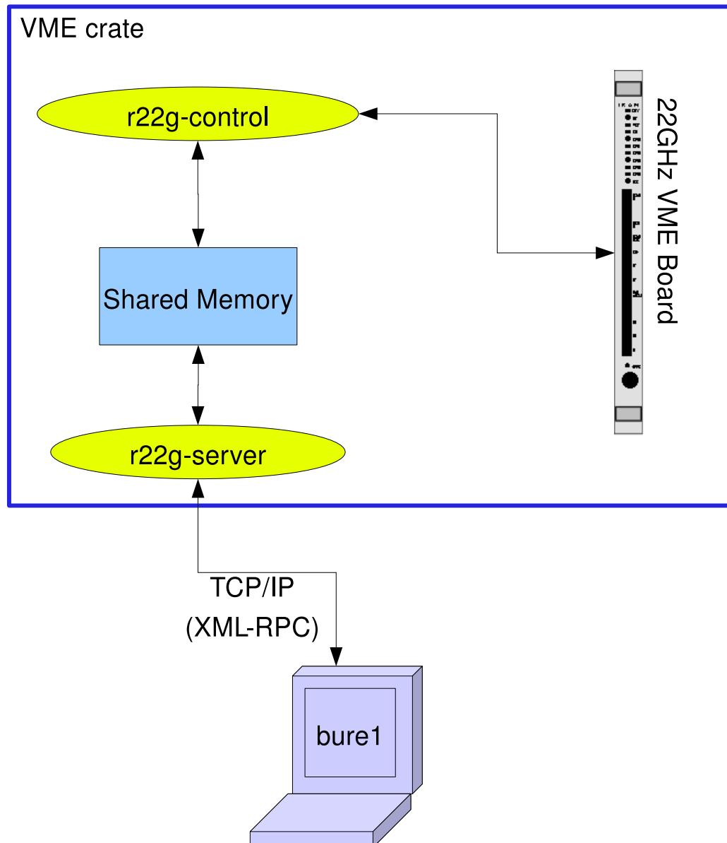
In each antenna cabin, **r22g-control** drives the 22GHz VME board and **r22g-server** handles the network requests from bure1.
