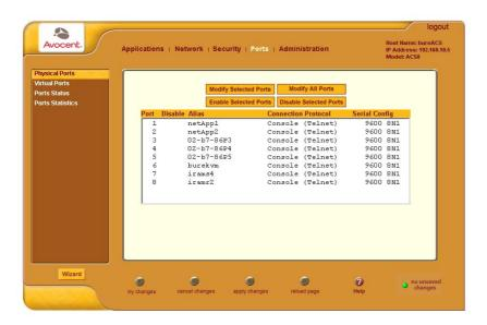
Click "wizard", you will come to "expert" mode. Choose Step 3/Port profile. Enable Telnet Console mode. Communication: 9600,8,N,1,No flow control. Click button "Apply changes"
