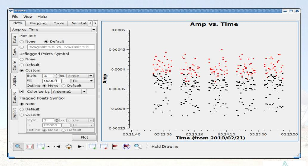
OMC-1. Plot of channel averaged data vs. time color coded by antenna1 for scan 10
