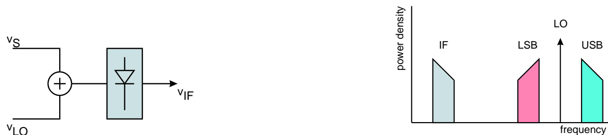
Figure 5.4: Frequency down-conversion by mixing. Left: schematic diagram. Right: representation in frequency space.
