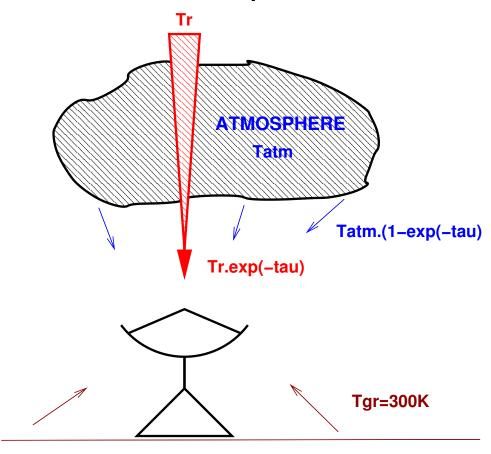
$$T = \alpha \left\{ T_R e^{-\tau_{\nu}} + (1 - e^{-\tau_{\nu}}) T_{\text{atm}} \right\} + (1 - \alpha) T_{\text{gr}}$$
