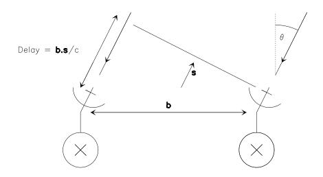
Precision: Spatial frequencies = baseline lengths projected in a plane perpendicular to the source mean direction.
