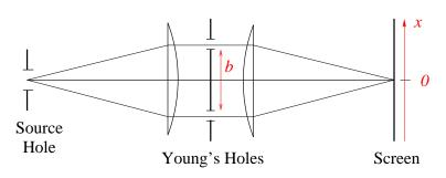
Lens  $\Rightarrow$  Fraunhofer conditions (*i.e.* Plane waves as if the source were placed at infinity).
