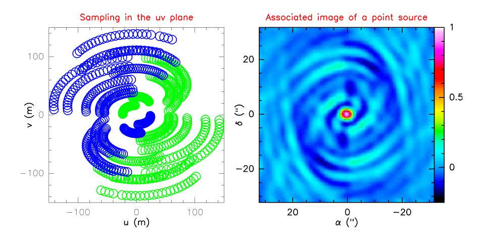
Precision: Spatial frequencies = baseline lengths projected in a plane perpendicular to the source mean direction.
