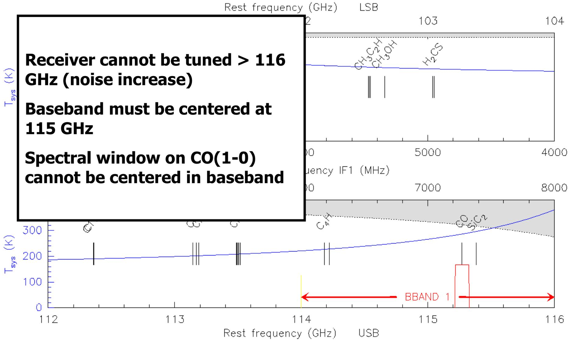
**Receiver cannot be tuned > 116 GHz (noise increase)**
