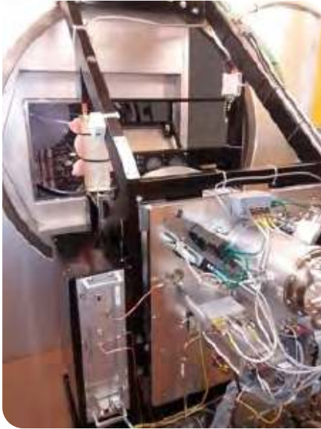
View of a dual-band receiver as installed on Antenna 10 in December 2021.
