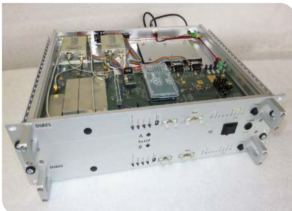
The optical roundtrip system is designed with the Laser transmitter and optical receiver located in the upper left corner.
