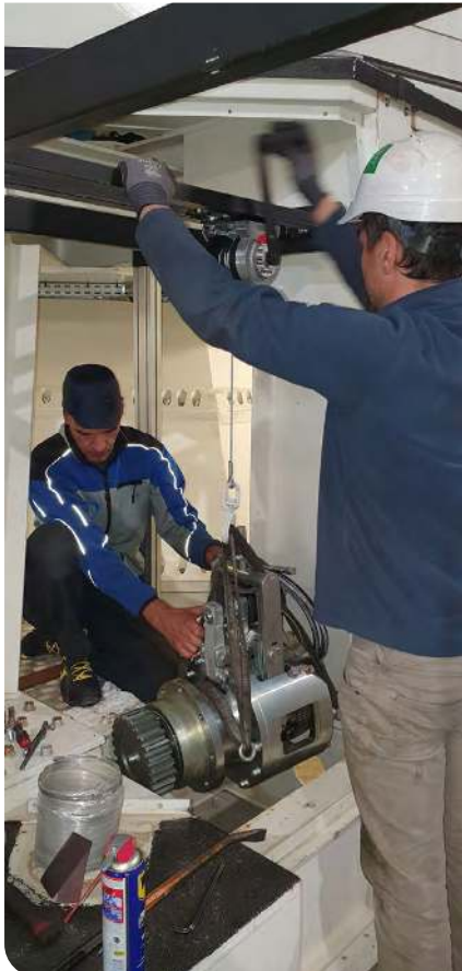
Left: Integration of the new braking device on Antenna 8.
