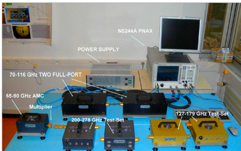
The three MVNA Test-Sets extenders with the AMC power source, the Agilent N5244A PNAX and the power supply.
