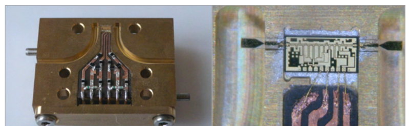
Left: LNA base block (cover block removed) showing the input and output waveguides and DC bias board. Right: IAF MMIC glued to LNA base block in between two waveguide-to-CPW quartz probe chips.
