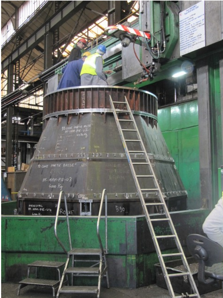
Machining and factory pre-assembly of the first NOEMA antenna mount.
