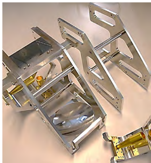
Support frames and optical components for the NOEMA receivers.
