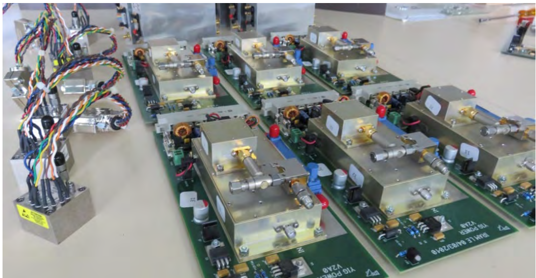
View of the new batch of LO1Ref modules during assembly. On the left: a set of YIG voltage-controlled oscillators.
