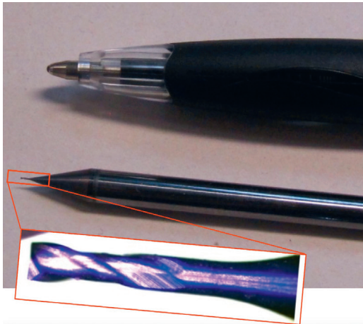
Cutter with 0.2 mm width and 1.0 mm length for the high-precision milling of grooves of the 2 mm band-pass filter block.
