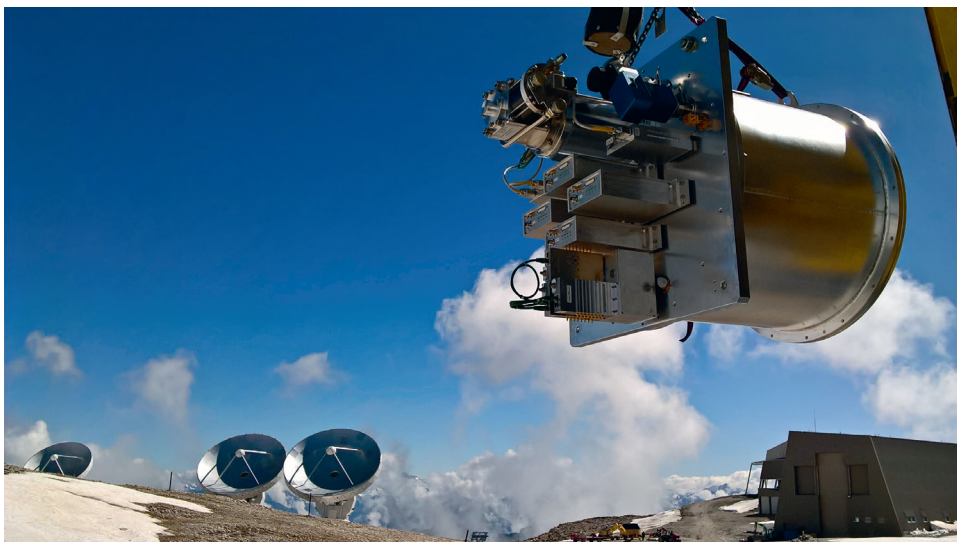
Top: NOEMA receiver assembly stages. The photos show the complex optical modules, mixers, and amplifiers positioning (left and center) and the full system closed in a cryostat (right) with four astronomical windows (Band 1 to 4), and two additional windows dedicated to calibration.
