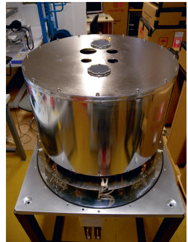
Top: NOEMA receiver assembly stages. The photos show the complex optical modules, mixers, and amplifiers positioning (left and center) and the full system closed in a cryostat (right) with four astronomical windows (Band 1 to 4), and two additional windows dedicated to calibration.
