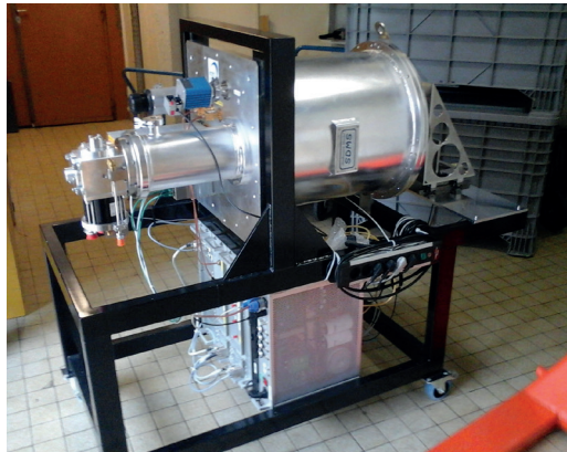
Dual-band receiver constructed by IRAM for the Max-Planck-Institute for Solar System Research.
