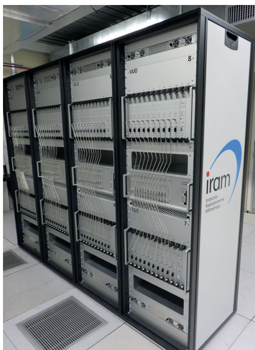
Front view of the full PolyFiX system. Each of the four cabinets is processing an 8 GHz sideband from the NOEMA receivers.
