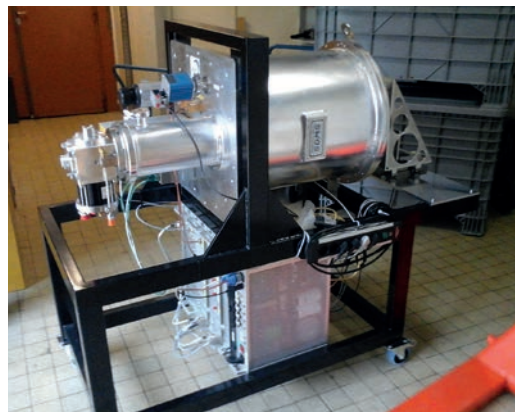
Dual-band receiver constructed by IRAM for the Max-Planck-Institute for Solar System Research.
