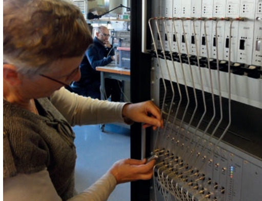
Technician performing system integration tests on a PolyFiX unit before its shipping to the NOEMA Observatory.
