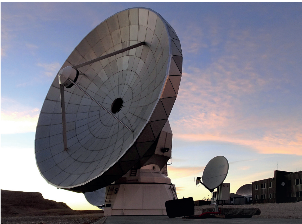
View of one of the two small commercial satellite dishes used for the phase monitoring project, installed at the Plateau de Bure, next to one of the NOEMA antennas.
