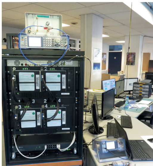
Right: The VLBI formatter board under test into the PolyFiX unit. (10GbE data link to the Mark6 through SFP+ optical transceivers on front, Intel Arria10 FPGA at the center of the board).
