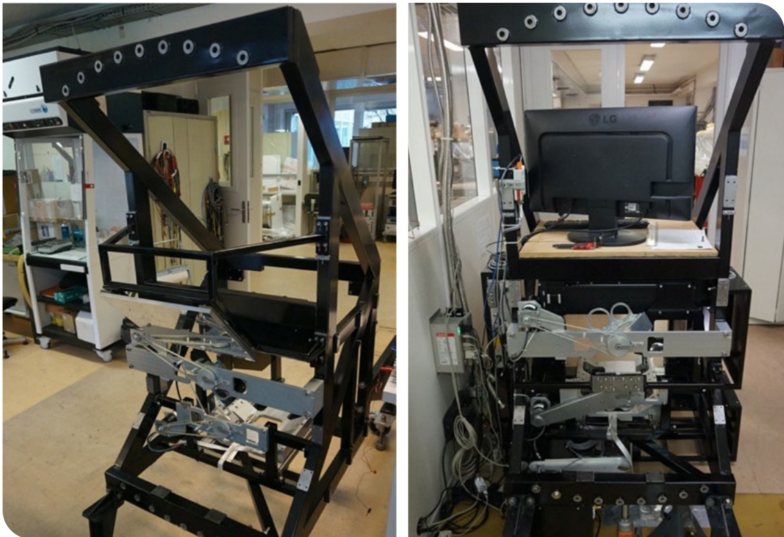
Two new frames called “chassis-A” were manufactured specifically for the dual-band mode of operation. They are partially integrated with the translation stages, optics and moving mechanism used for the calibration.
