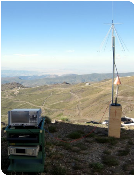
Setup used for the measurements of radio-frequency interferences in the IF bandwidth of the receivers.
