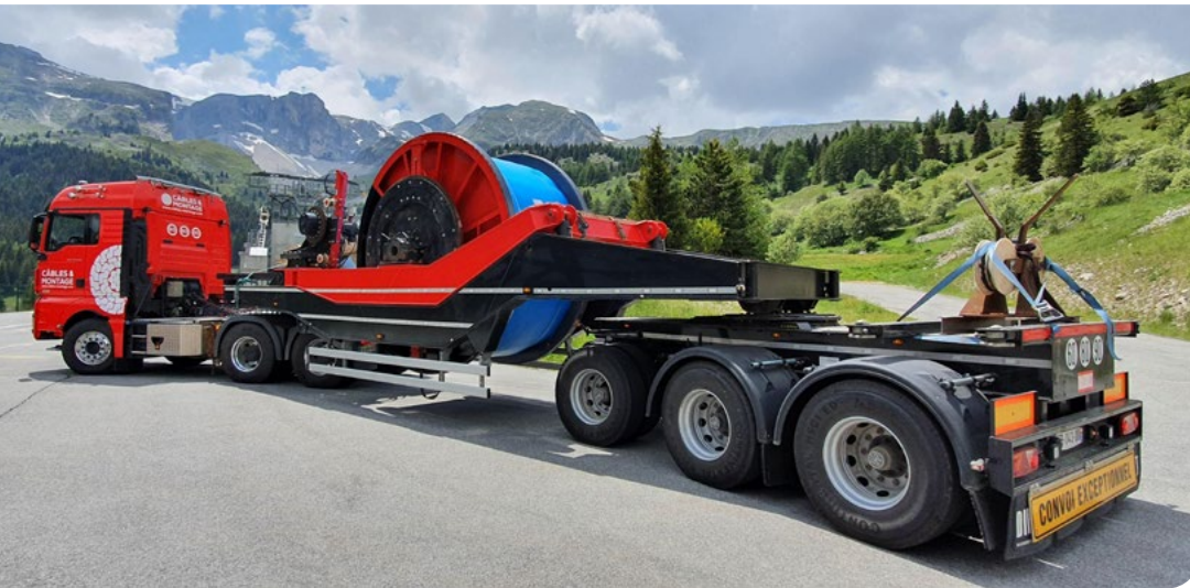
Transport of the new track rope by exceptional convoy.
