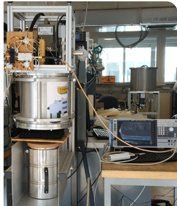
Test setup, with the cryostat at the middle left. A new spectrum analyzer with noise figure measurement capabilities was purchased in 2020 allowing to noticeably speed up testing.
