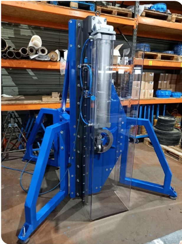
Test-bed of the emergency brake system to be installed on NOEMA antennas.
