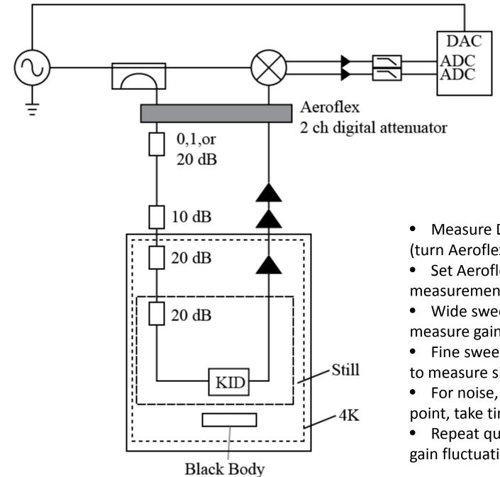
Measure DC offset (turn Aeroflex to max attenuation)
