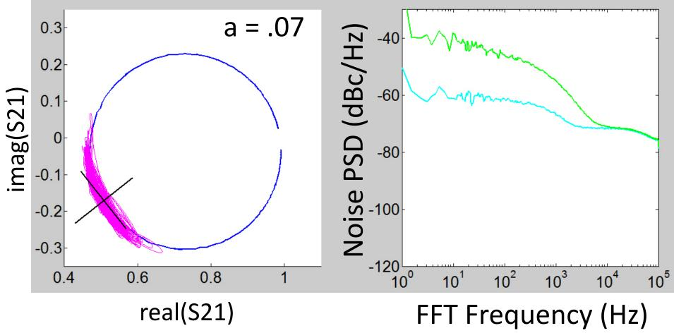
At low powers, noise has significant curvature
