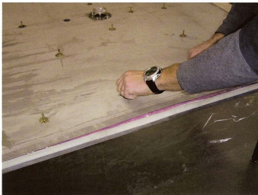
Fig. 4.4: Back skin of one of the MediaLario panels. The glue (violet colour) can be seen between the inner structure and the back skin surface.
