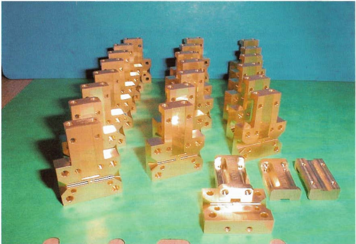
Fig. 5.14: A series of 2SB mixer for the ALMA band7.
