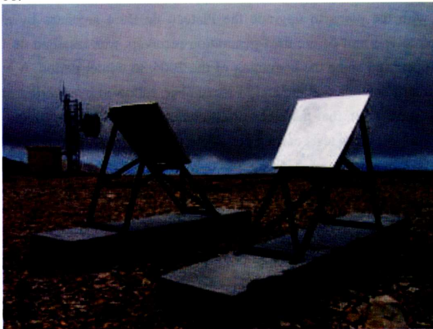
Fig. 4.8: Two ring 4 MediaLario panels oriented North and South mounted on their unsheltered test platforms.
