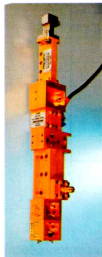
Fig. 5.10: Left Side: Full-electronic local oscillator for the 283-365 GHz band. Only the waveguide elements are shown; not shown are the lower frequency, coaxial elements: YIG oscillator 15.7-20.3GHz, and doubler. Right Side: Comparison of the noise performance of the same 300GHz band SIS mixer, pumped either by a traditional Gunn-tripler, or by the full-electronic local oscillator. The millimeter-wave bandpass filters developed for this project are a key element of the noise performance of the LO. (Int.J.I.R.MM.Waves, in press).
