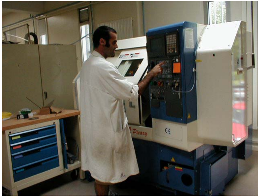
Fig. 5.12: The new cnc controlled lathe “TAKAMAZ” for lenses and horns
