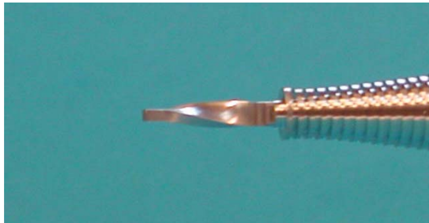
Fig. 5.13: A “twisted” horn design for the next generation of Plateau de Bure receivers.
