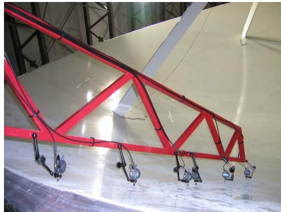
Fig. 4.7: System of 6 micrometers measuring the panels of rings 5 and 6 of antenna 2
