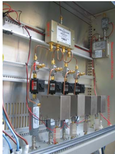
Fig. 3.3: A new IF processor for VLBI, VESPA and the 1MHz and 100kHz filter banks.
