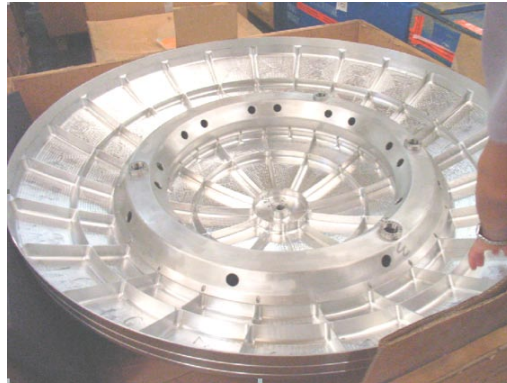
New sub-reflector for the Plateau de Bure 15-meter antenna.
