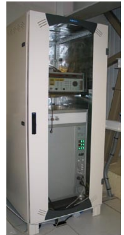
The EFOS-38 hydrogen maser in its temperature controlled rack, which also houses the Racal Dana frequency generator. The rack improves the stability of the internal regulation of the maser, which is monitored over 42 of its vital operating parameters. This allows to optimize the maser performance, and to fully exploit the capacities of this frequency standard, which was designed to allow VLBI observations up to 350 GHz.
