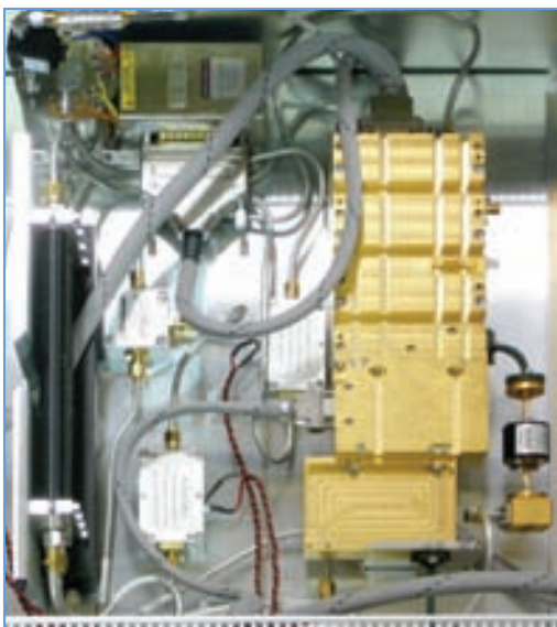
Above: local oscillator box in current use on IRAM telescopes (RF part only). Below: New LO with no moving parts (RF part only). Note the lower parts count and simpler layout.
