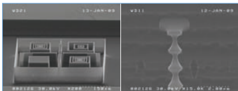
Above: Micro- and Nanostructures as defined by silicon micro machining employing micro lithography and plasma etching.
