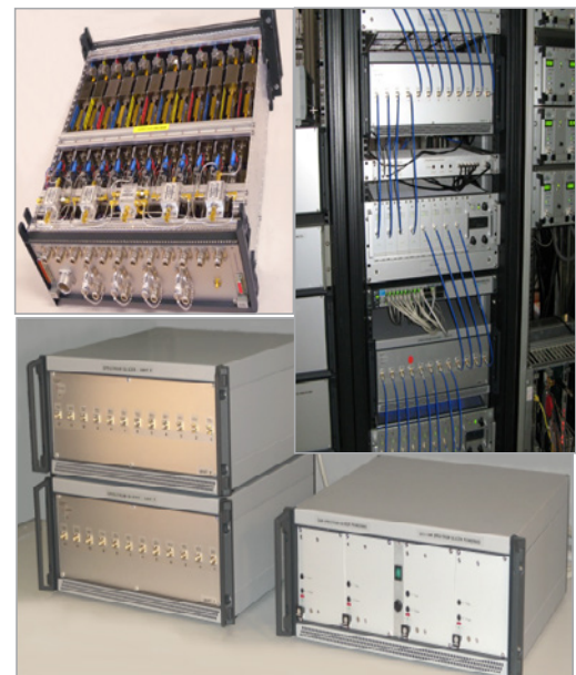
Top left: One of the two spectrum slicer racks (with cover removed) including 12 sub-units. Bottom left: Spectrum slicers and common power unit. Right: FFT backends installed on the 30 m telescope. Three FFT racks (each including eight FFT units) and two spectrum slicer racks are connected through coaxial cables.
